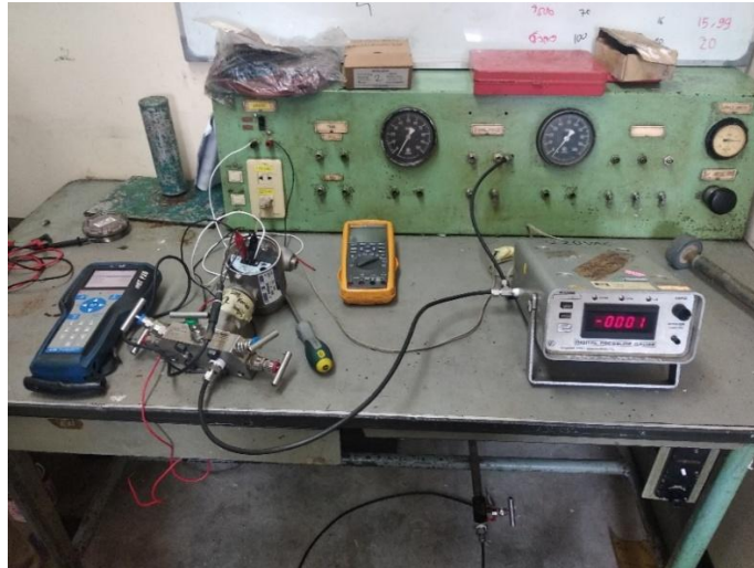
Gambar 4.16 Proses Kalibrasi Transmitter Temperature RTD Pt100
